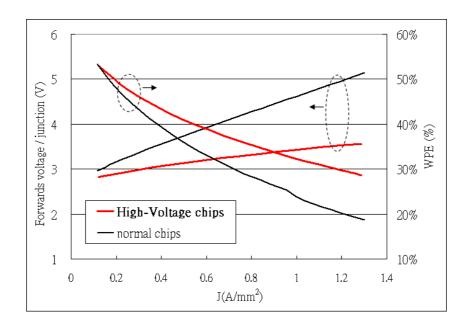
HV chips have higher WPE and lower forward voltage as compared to normal power chips with the same chip size.
